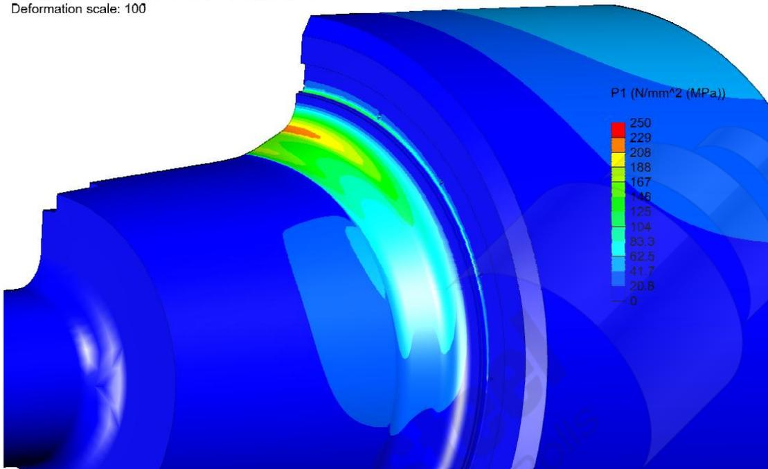
FEA plots showing a typical example for the location and depth of peak bending stress developed in a back up roll
