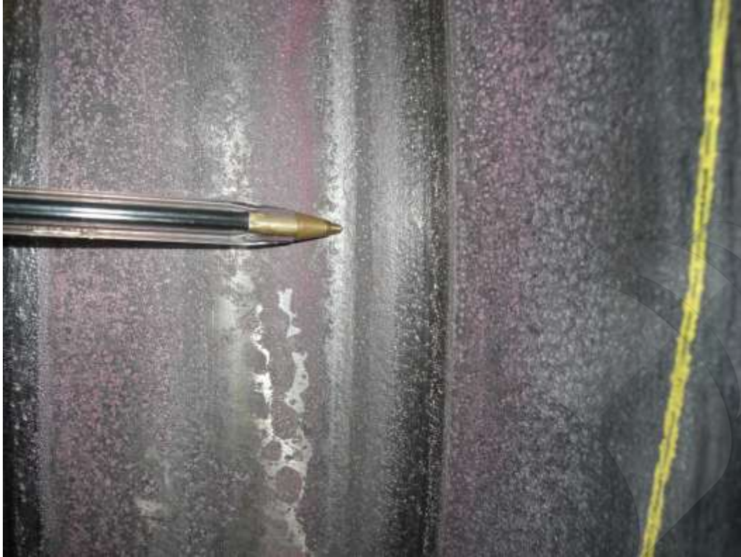
Figure 4 Extensive corrosion pitting of a back up roll barrel face radius.
